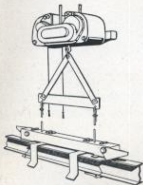
Lowerator powered with a vertical electric hoist.
