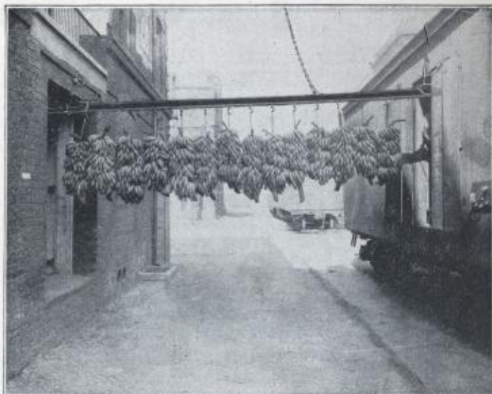
Removable section of track with car hook hastens banana unloading
